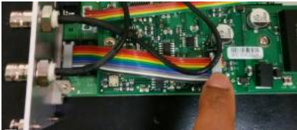
The Second 10-pin Header connector
