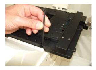
Next move the stage, again with the controller joystick, to the left until the plate cut out is aligned over the microscope mounting screw hole position. This will be near the leftmost position. Install the third mounting screw.
