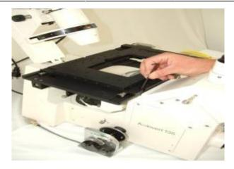
With the controller powered on move the stage, using the controller joystick, to the right until the plate cut out is aligned over the microscope mounting screw hole position. This will be near the rightmost position. Install the second mounting screw.
