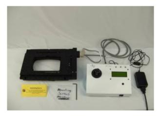
Remove System from packaging. Remove the stage locking bolt and connect stage controller with the provided cable. Connect the power brick to controller and turn on the system. Then, place the stage onto microscope stand.
