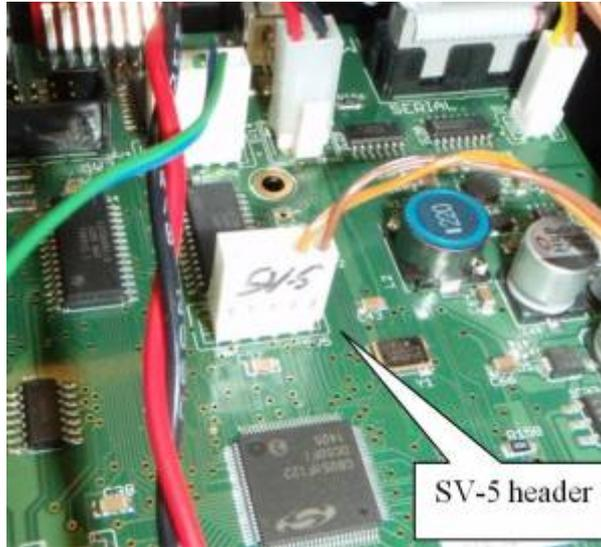
Once the header is installed and the rest of the cabling to the stage and the system is connected normally, then test the function of the Joypod in X, Y, and Z directions and test the function switch, if it has a function applied to it.
