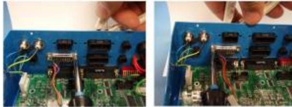
STEP 6: Next, check to see that the replacement Z- Linear Encoder Header works before mounting the header by connecting the linear encoder to the Z- Linear Encoder Header at one end and to the SV-2 mother board port at the other. Next turn on the controller in Z- L.E. mode, (dip switch #6 down), and check the motion of the Z drive.
