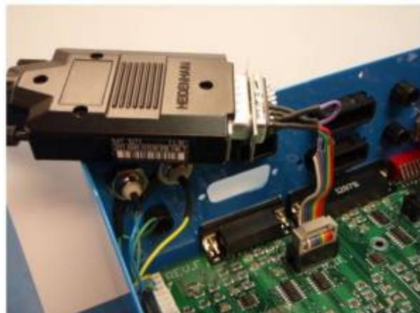
If the system performs correctly then the Z- Linear Encoder Header can be mounted into the case in the reverse order it was removed. Next if all the wires are routed away from the joystick and that the case is clean and clear of foreign debris, (screws, washers, etc.). The lid can now be screwed back on with the six 4-40 screws in reverse order of step 2. Once the lid is screwed on jiggle the case to make sure that nothing is rattling around inside the case.
