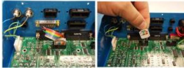
STEP 5: Using a 3/16" socket driver and pliers remove the two jack screw nuts and the two lock washers from the back of the Z-Linear Encoder Header. Remove any parts that fall inside the controller.
