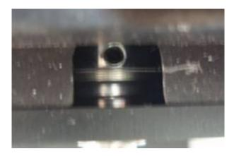
Step 6: Finally adjust the software offset to center the wheel with the opening in the body. The instructions are in the filter wheel manual and reprinted here.
