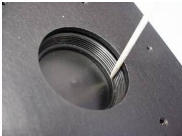
ASI FW 1000 filterwheels use a split retaining ring to hold filters, as shown above.
