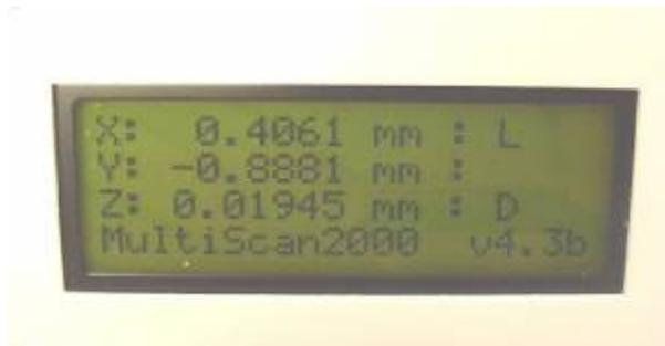
Check the operation of the limit switch by slowly moving the stage toward the end of travel. When a limit is reached, the motion will be terminated and the letter “U” or “L” will appear on the LCD screen showing that the limit is in force
