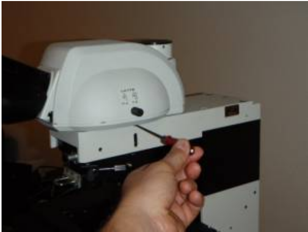
Figure 12. Install trinocular head assembly back on the microscope.
