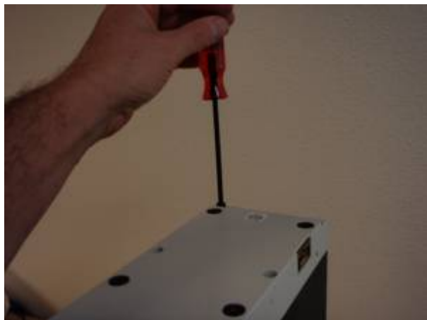
Figure 7. Location of four screws that remove / secure trinocular head base
