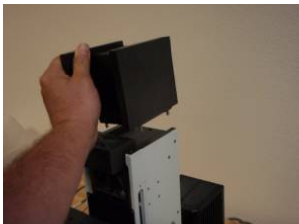
Figure 8. Installing the trinocular spacer, note alignment pins
