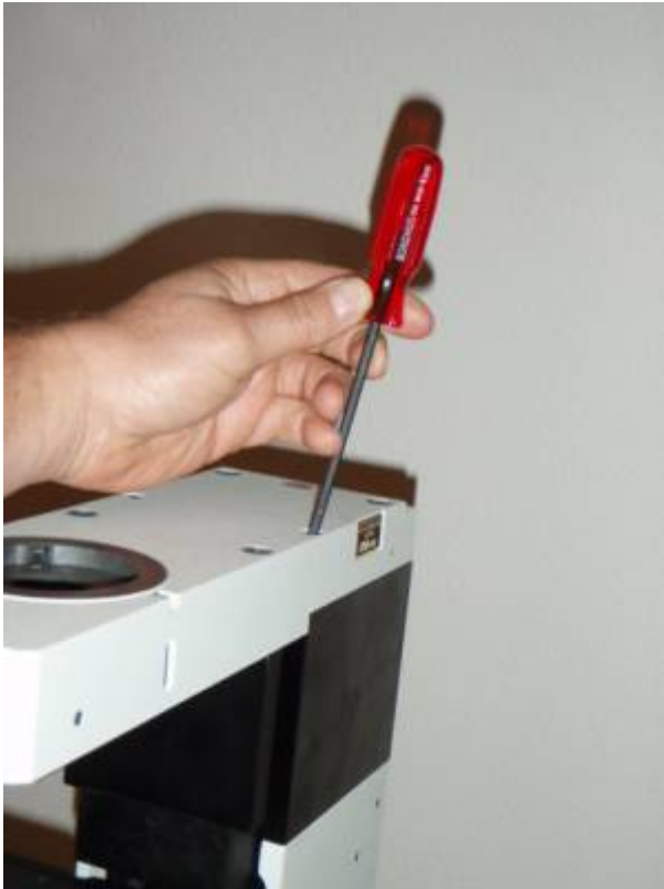
Figure 11b. Installing the trinocular mount back onto the microscope body
