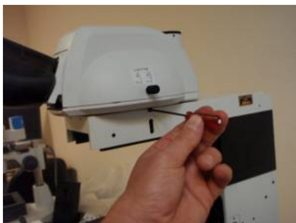
Figure 6. Location of set screw to remove / secure trinocular head
