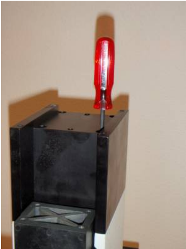
Figure 9. Use the 4 mm Allen wrench to tighten the 4 each 5 x 40 mm cap screws that secure the trinocular adapter to the microscope body
