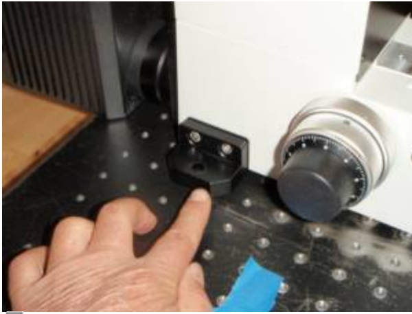
Figure 2. Standard Nikon adapter plates mount onto the microscope body at four points. Please refer to the Nikon manual for information on mount these plates
