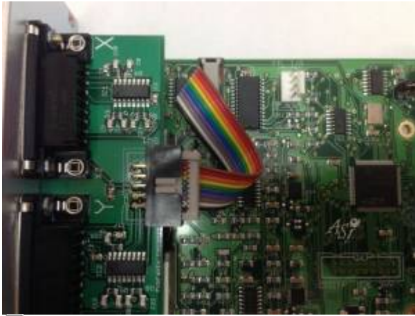
Figure 3 LE Buffer card and Two axis card are connected with a 10pin straight ribbon header connector
