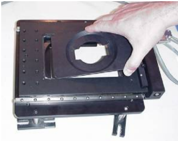
Figure 1. Slide the insert from the side of the stage that does not have the spring clips.
