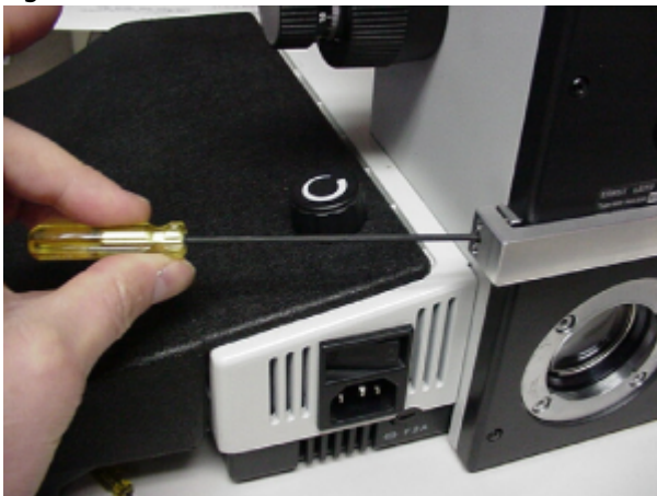
Figure 11: Use the 5/64" Allen Wrench to tighten the Base plate clamp at a point where the vertical adjustment screws are midway in the slots
