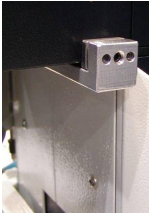
Locate the Heidenhain encoder and the encoder clamp. Use the 3/32 Allen wrench to insure that the screw on the side of the encoder clamp is loose. Install the encoder clamp across the rear throat of the microscope as shown. Use the 5/64 inch Allen wrench to tighten the set screw located on the opposite side of the silver press bar. This will cause the silver press bar to press against the microscope and will hold the encoder holder securely in place.
