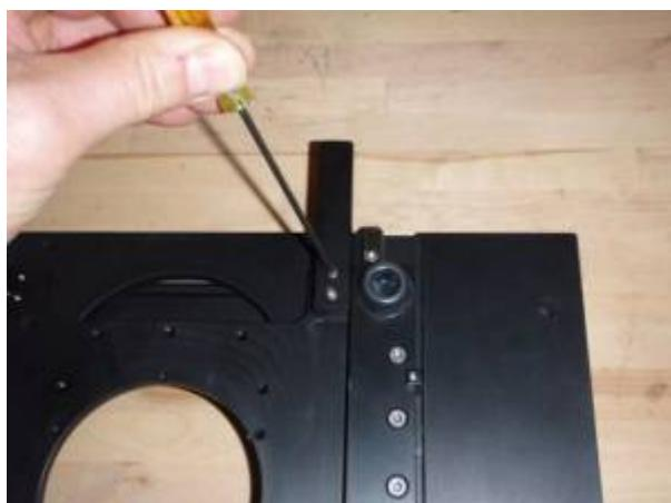
The linear encoder stop mounts onto the bottom of the stage as shown in the above photos
