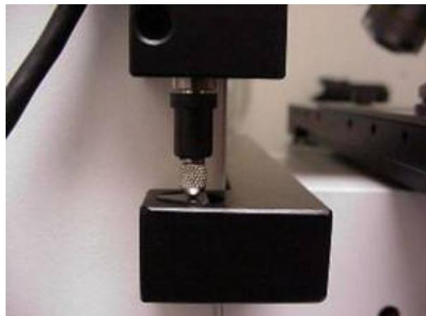
Bring the stage up to the correct focal position for the common objectives used. Position the encoder & encoder clamp so that the ball on the end of the encoder's plunger mates with the triangular carbide plunger stop. Insert the encoder into the encoder holder & slide the encoder down until there is about 1 to 3 millimeters worth of upward travel left on the encoder's plunger. Hold the encoder in place & use the 3/32 inch Allen wrench to tighten the screw to secure the encoder in place.
