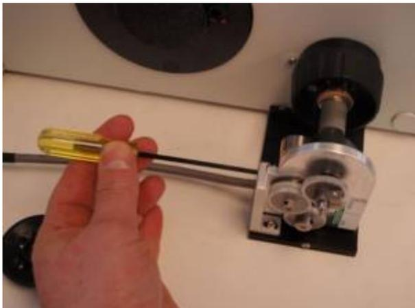
Figure 9. Use the 7/64" Allen wrench to loosely tighten the two vertical adjustment screws that were loosened in figure # 5.
