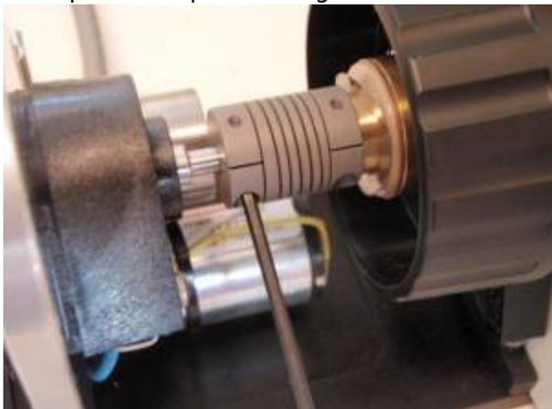
Figure 8. Use the 5/64" or 2 mm Allen wrench to securely tighten the flex coupler onto the ASI Z drive shaft. Please note that this screw must be securely tightened to prevent slippage.
