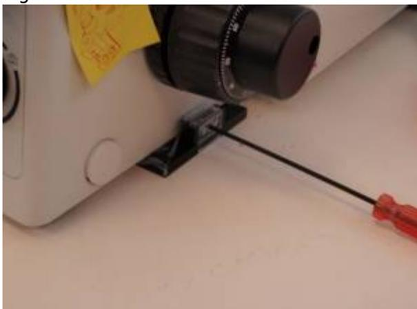
Figure 7d. As shown in the above photos install the Z-drive onto the base plate by sliding the drive shaft into the flex coupler, and installing the horizontal adjustment screw that was removed in figure # 4. Use the 7/64" Allen wrench to lightly tighten this screw. Please note that the base plate may need to be moved slightly to align everything correctly. Use the 5/64" Allen wrench to tighten the base plate camp on the right side of the microscope as shown.
