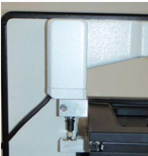
The procedure outlines the steps necessary to install and align the ASI Heidenhain linear encoder onto the Leica/Leitz LABORLUX S series microscopes. The linear encoder mounts to the upper front of the microscope's armature via an encoder clamp. The linear encoder has a plunger that depresses into the encoder as the focusing position is moved. The plunger tip mates with a plunger stop that is attached on the microscope's carrier.
