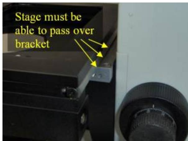
Locate the plunger stop and position it on the stage carrier so that the metal press bar is on the right side and the round carbide plunger stop is on the left side of the stage carrier as shown in above.
