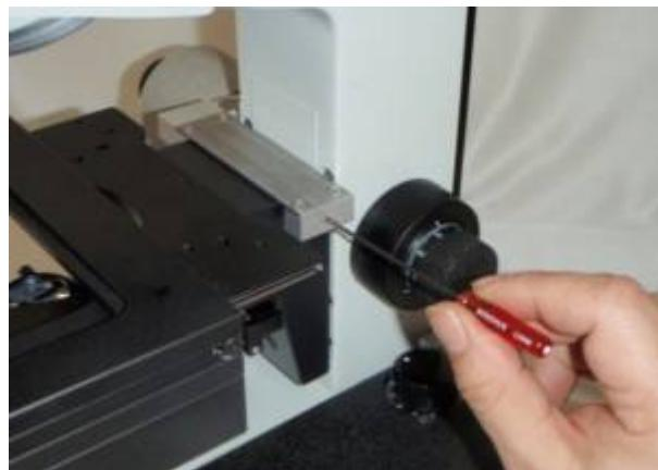
Once correctly positioned use the 1.5mm Allen wrench to tighten the set screw located on the opposite side of the silver press bar. This will cause the silver press bar to press against the microscope and will hold the plunger stop securely in place.
