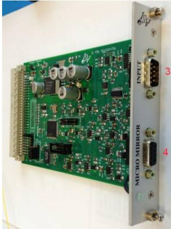
MicroMirror Drive Card. Connect 4 to MicroMirror Scanner body thru a DB9 straight cable. 3 is the input to accept analog signals. Analog input range is 0-5Volts.
