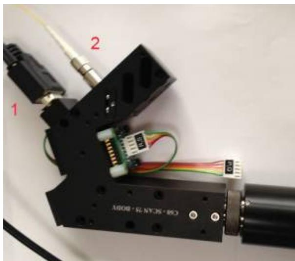
MicroMirror scanner body. The DB9 connector (1) connects to the MicroMirror Drive Card thru a DB9 straight cable. 2 is the fiber optic coupler. As shown in the picture, MicroMirror is connected to drive card as R and S axis. Newer scanners have the fiber connector on the end of the scanner body.
