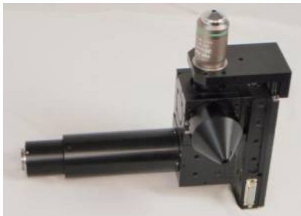
MIM3-OSM25-2PII w/ TN200-MMC inverted scope
