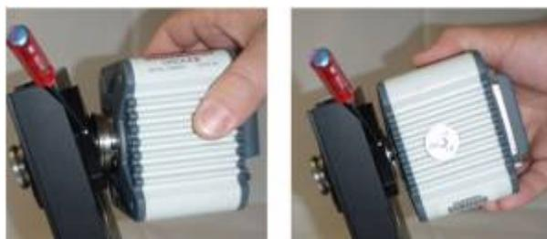
Tighten the three retaining set screws. They are 120 degrees apart from each other.
