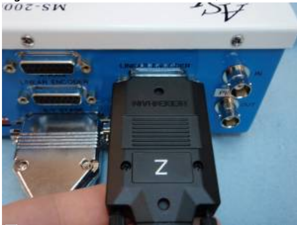
Figure 18. Z-Axis Linear Encoder plugged into controller
