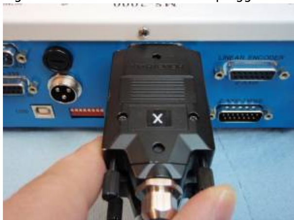
Figure 13. X-axis Linear Encoder plugged into controller. (top plug).
