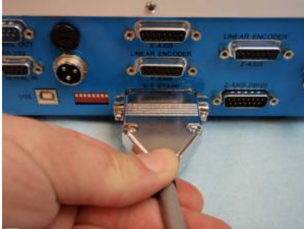
Figures 8. XY Stage cable plugged into controller
