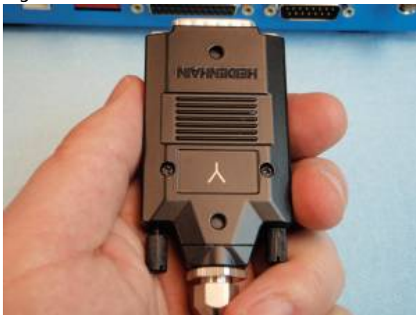
Figure 10. Y Axis Linear Encoder plugged into controller. (bottom plug).
