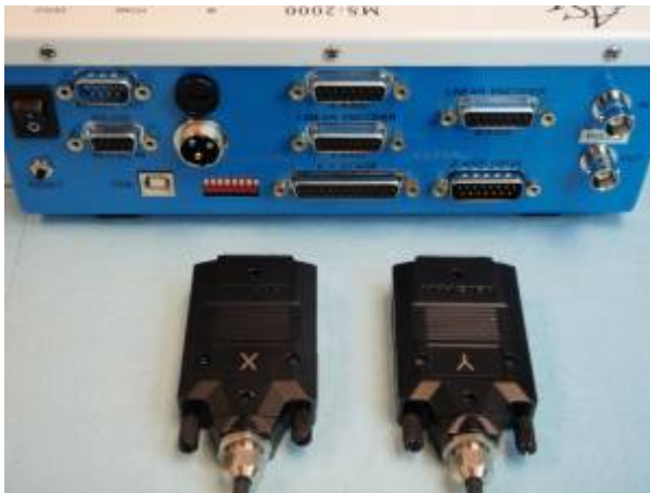
Figure 9. XY Linear Encoder Cables and the back of the MS-2000 controller.
