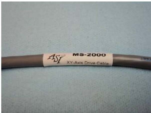
Figure 6. XY Stage cable, controller end label
