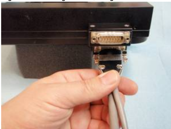
Figure 4. X-axis cable connects to bottom stage plug.
