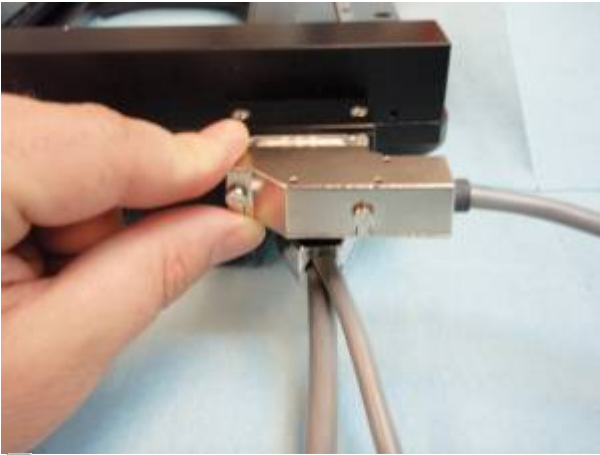
Figure 5. Y-axis cable connects to top stage plug
