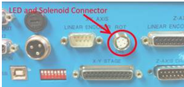
Location of 4-Pin HiRose Connector and TTL out on MS2000 and MFC2000
