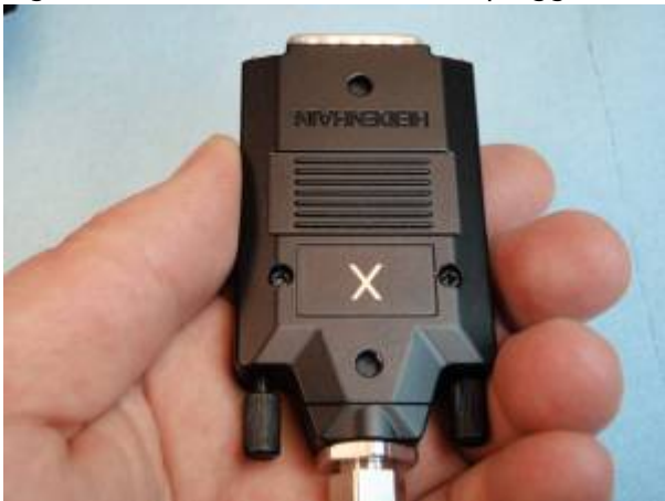
Figure 12. X-axis Linear Encoder plugged into controller. (top plug).
