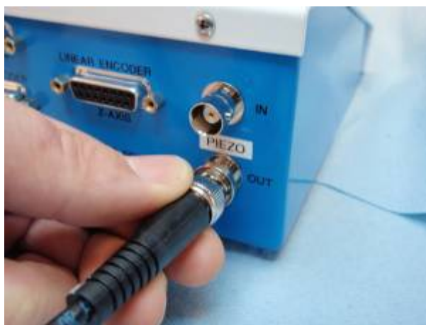
Figure 25 Piezo Out Plug on MS-2000
