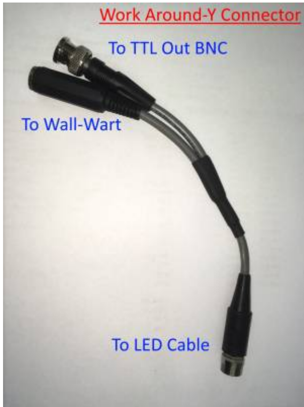
Work Around Y cable
