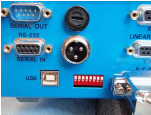
Figure 23. Power Connector on MS2000
