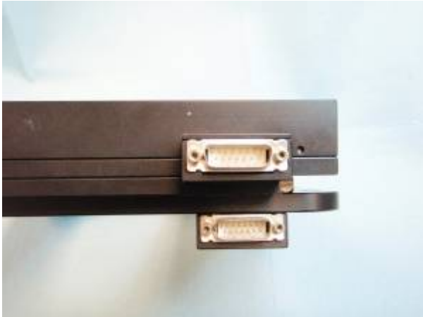
Figure 2. XY Stage connectors on stage
