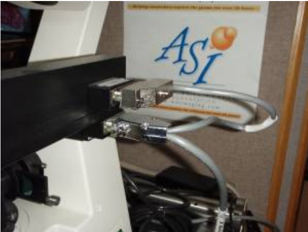
Figure 6. XY Stage cable, controller end label
