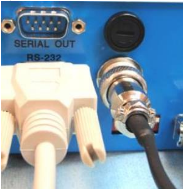
Figure 24. Power Plug connected to MS2000
