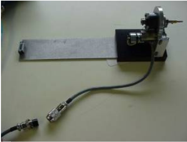
Figure 14. Z-Drive and Z-Drive cable connected
