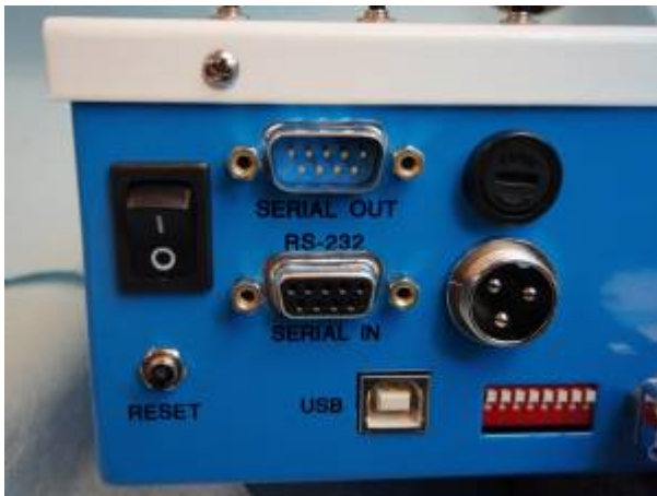
Figure 19 Serial-In Plug on MS-2000
