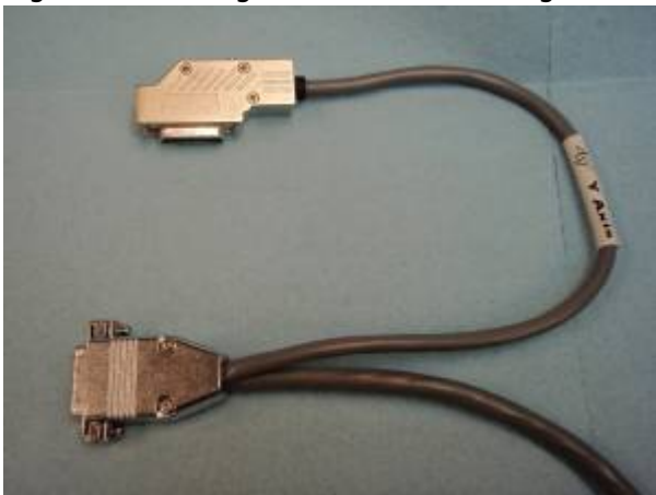
Figure 3. XY Stage cable, stage end.
