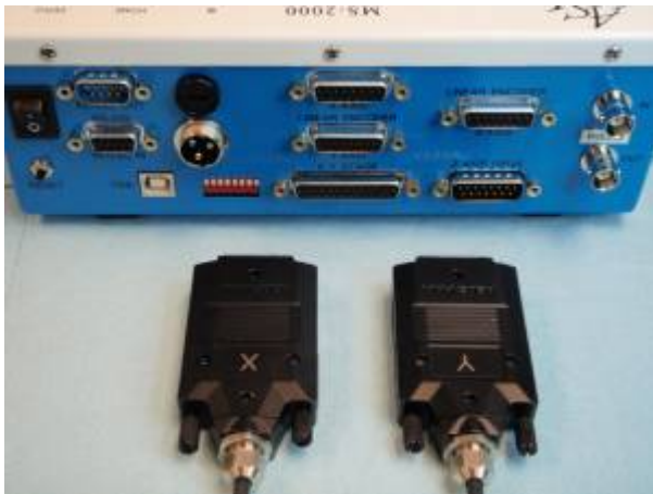
Figure 9. XY Linear Encoder Cables and the back of the MS-2000 controller.
