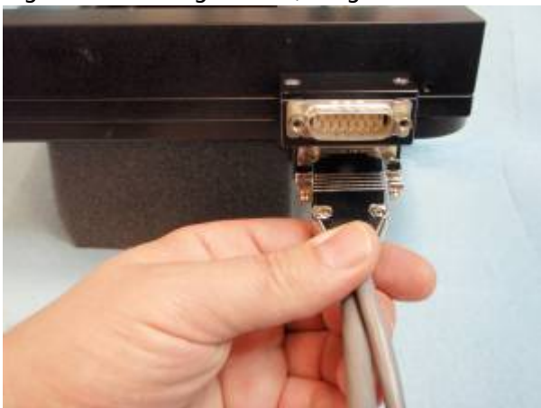
Figure 4. X-axis cable connects to bottom stage plug.
