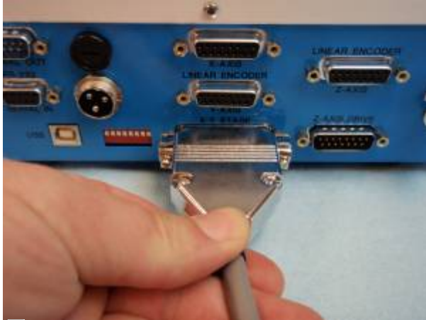
Figures 8. XY Stage cable plugged into controller
