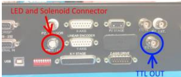
Location of 4-Pin HiRose Connector and TTL out on RM2000
