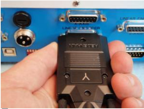
Figure 11. Y Axis Linear Encoder plugged into controller. (bottom plug).
