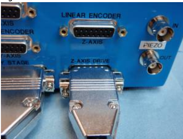
Figure 16. Z-Drive cable connected at controller end.
