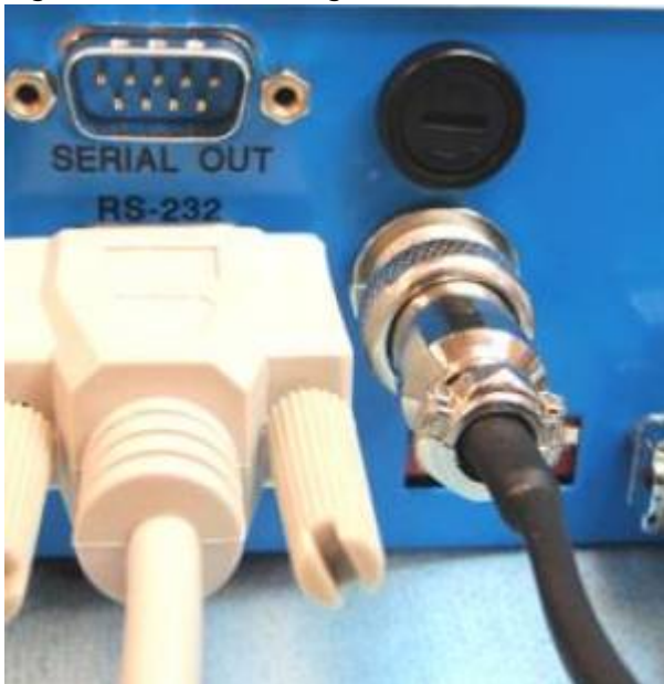
Figure 20 Serial-connected on to MS-2000
