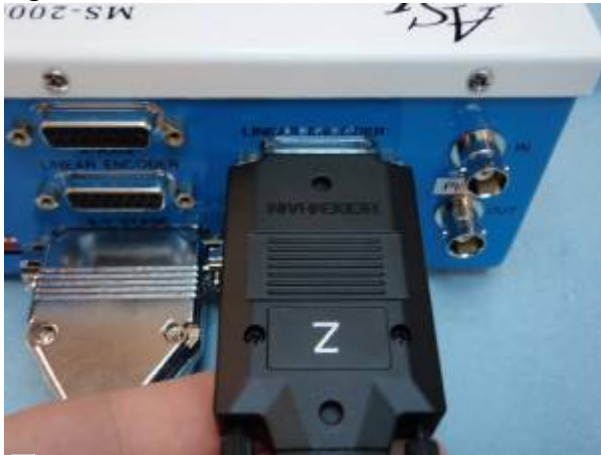
Figure 18. Z-Axis Linear Encoder plugged into controller
