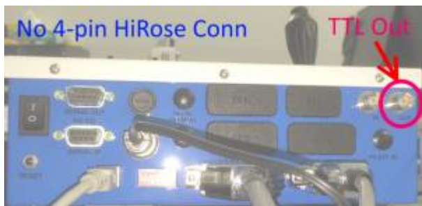
Controller with no HiRose Connector. However TTL Out is always present.
