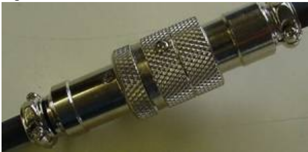
Figure 15. Z-Drive and Z-Drive cable connected
