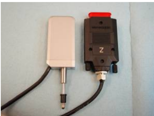
Figure 17. Z-Axis Linear Encoder and Z-Drive cable
