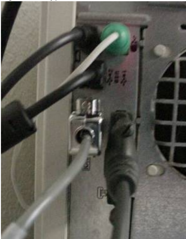
Figure 22. Serial cable connected
