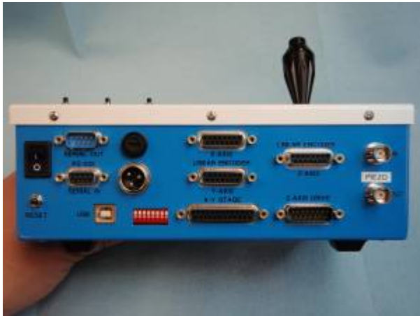
Figure 1. Back of MS-2000 controller with all options available
