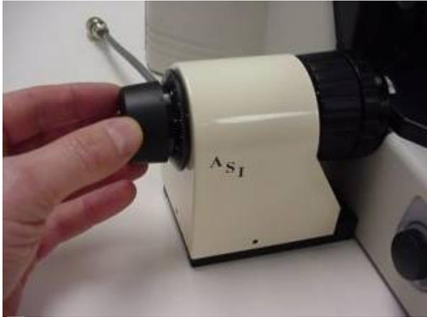
Figure 13: Installing cover and focus knob
