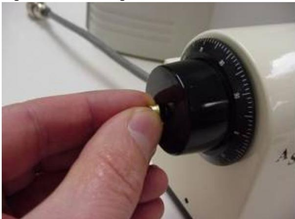
Figure 14: Installing cover and focus knob
