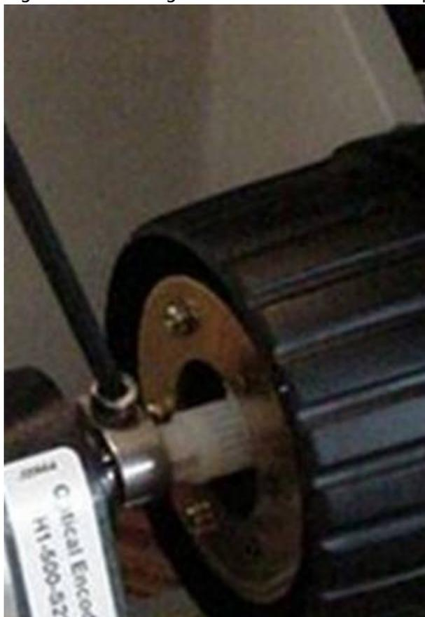
Figure 8: Tightening drive shaft clamp
