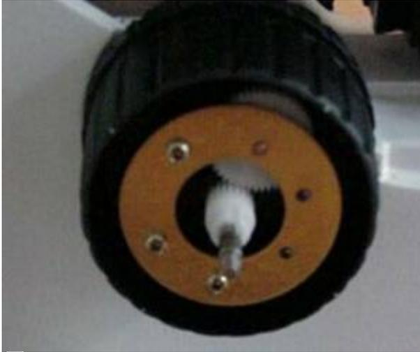
Figure 3: Pull knob straight off to expose shaft - Do not twist.
