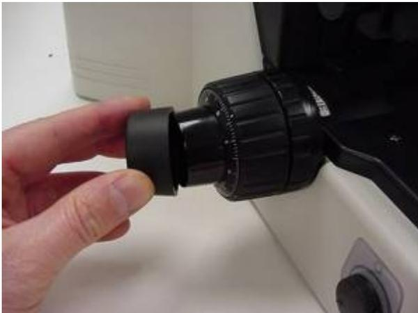
Figure 1: Pull off rubber boot
