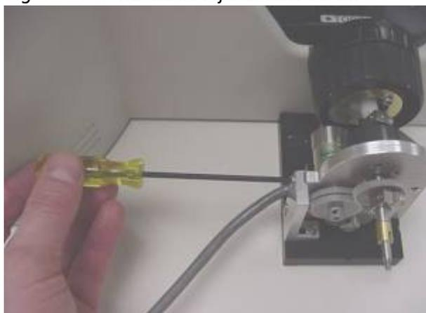
Figure 10: Vertical Adjustment screws
