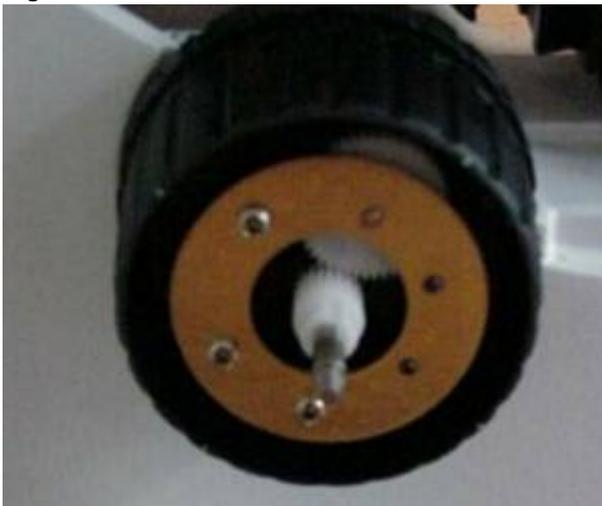
Figure 3: Pull knob straight off to expose shaft
