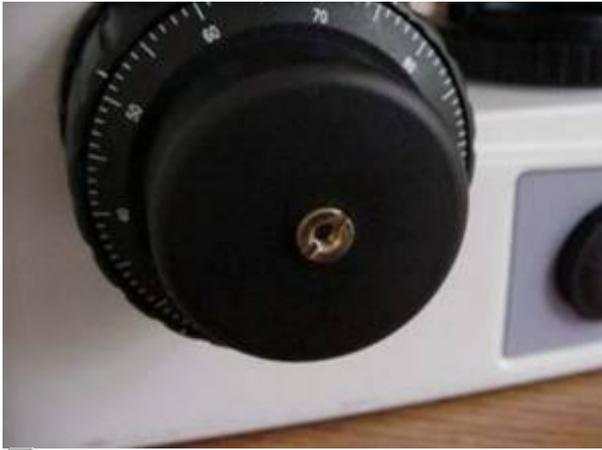
Figure 2: Use screwdriver to remove nut
