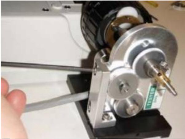
Figure 8: Secure but do not tighten adjustments
