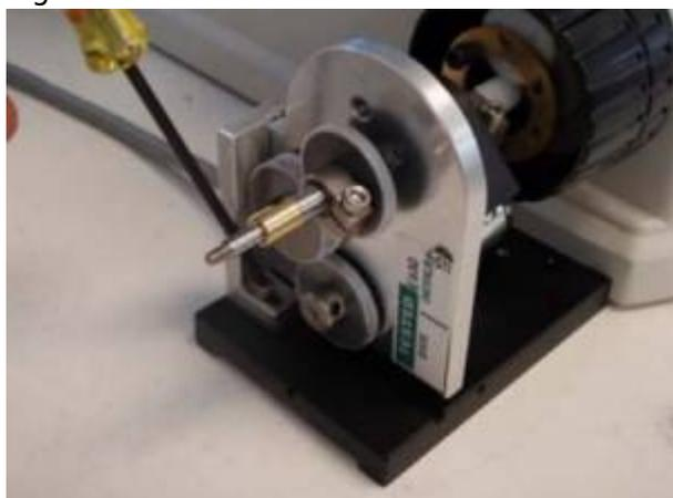
Figure 7: Base plate must be against scope
