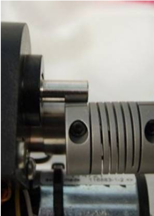
Coupler accepts about 4 mm of the drive shaft.
