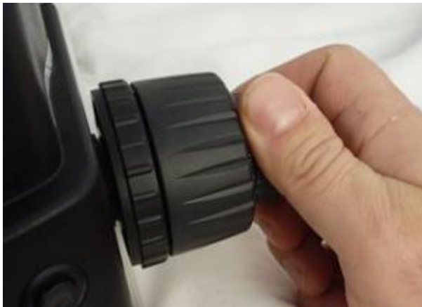
Hold the inner fine focus knob on the right hand side.
