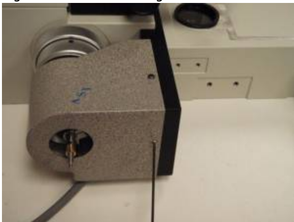
Figure 10c: Secure using 2mm Allen wrench
