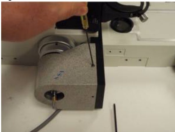
Figure 10b: Secure using 2mm Allen wrench
