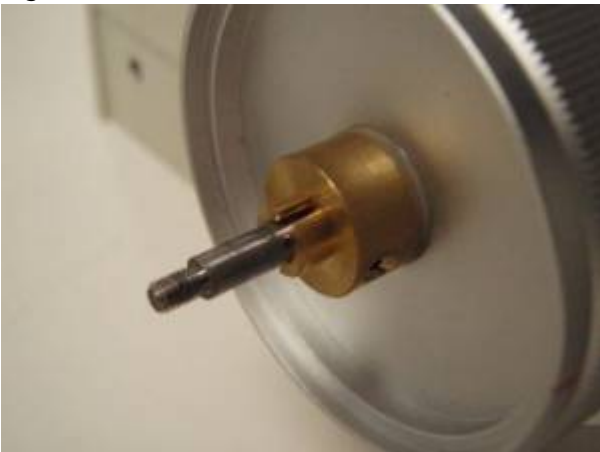
Figure 2: Pull knob straight off to expose shaft
