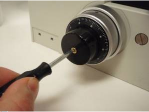
Figure 1: Use screwdriver to remove nut
