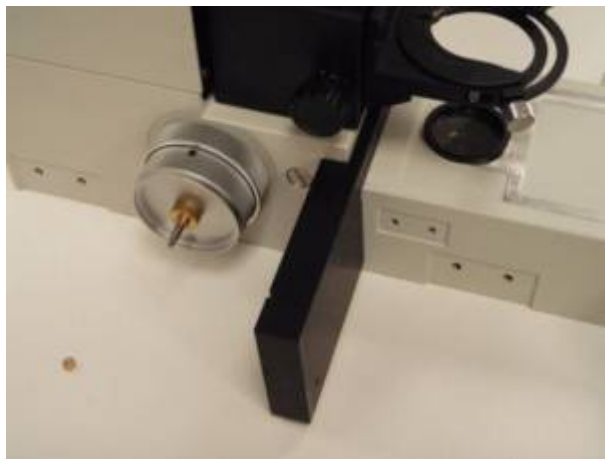
Figure 4b Install baseplate , bute leave the base plate clamp loose at this time
