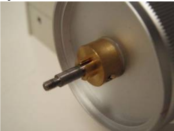
Figure 2: Pull knob straight off to expose shaft
