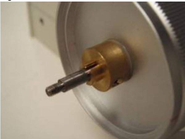
Figure 2: Pull knob straight off to expose shaft
