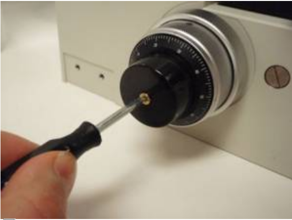
Figure 1: Use screwdriver to remove nut
