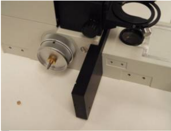
Figure 4b Install baseplate , but leave the base plate clamp loose at this time
