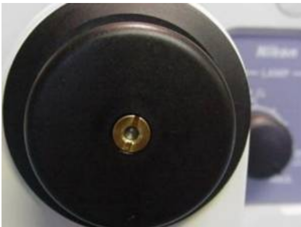
Figure 1: Use screwdriver to remove screw, and pull knob straight off. Do not twist
