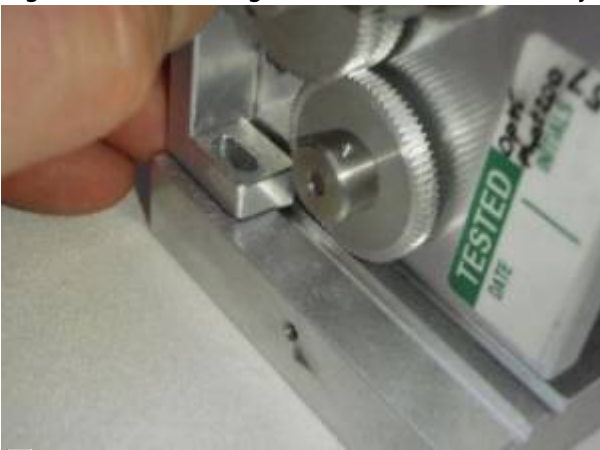
Figure 7b: Installing Z-drive. Note tab on adjustment bar slides into notch on base plate.
