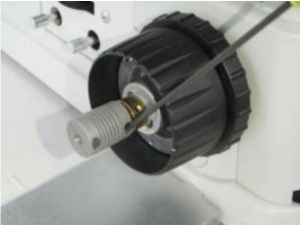
Figure 3: Use Allen wrench to secure flex adapter on microscope fine focus shaft.
