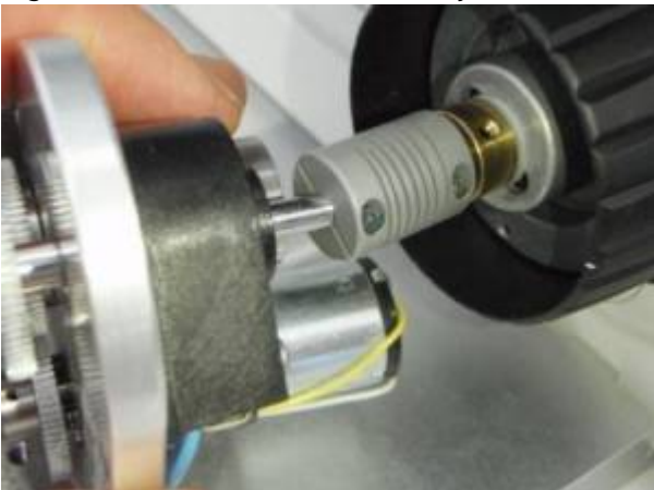
Figure 7a: Installing Z-drive. Note tab on adjustment bar slides into notch on base plate.
