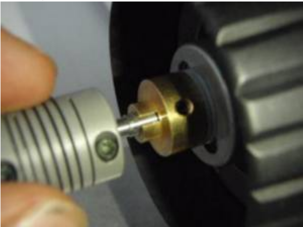
Figure 2b: Locate flex adapter & mount so that tabs cut into flex coupler mate with the notches on the brass piece
