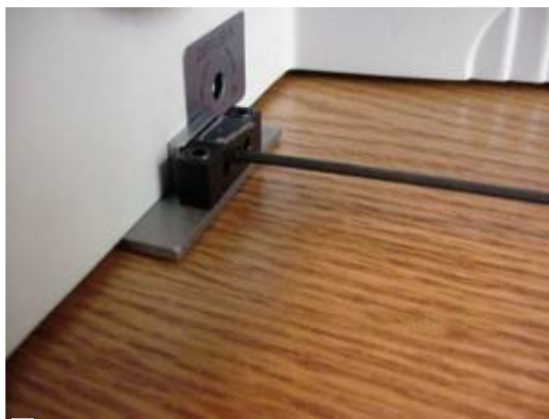
Figure 9: Tighten Baseplate set screw
