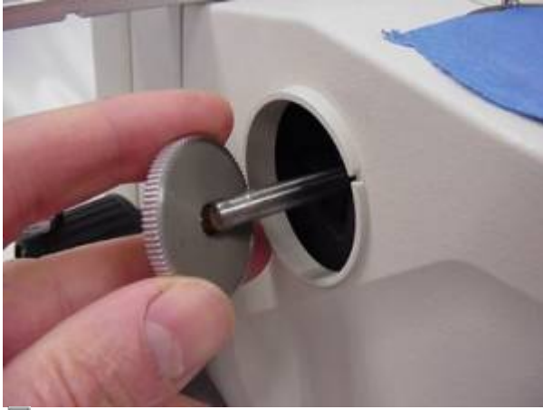
Figure 15. Installing zoom gear & spacer onto zoom shaft
