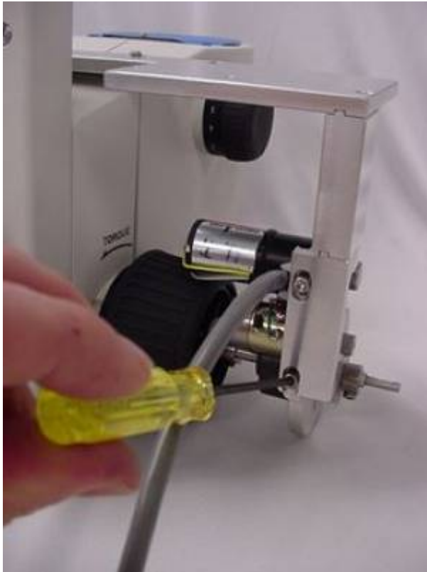
Figure 13. Tighten the vertical adjustment screws
