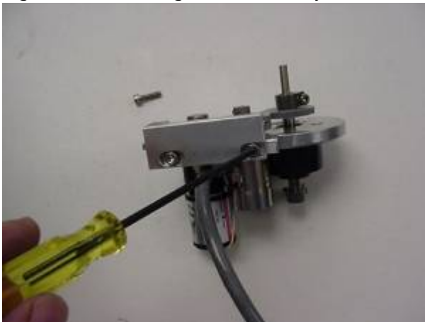
Figure 3. Z drive removed and vertical adjustment screws being loosened
