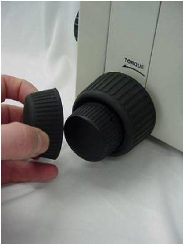
Figure 1a remove left fine focus & zoom knobs
