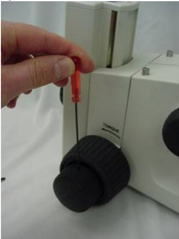
Figure 1b remove left fine focus & zoom knobs
