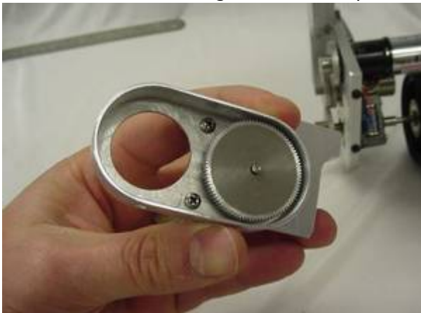
Figure 17. Located the zoom drive & cover and install it as shown in figure 14 so that the gears mate.
