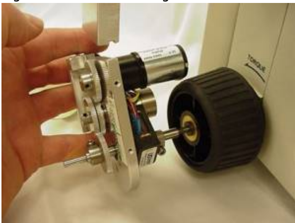
Figure 10. Install Z-drive over fine focus shaft.
