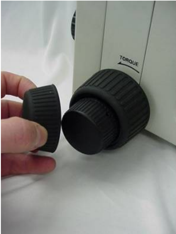
Figure 1a remove left fine focus & zoom knobs
