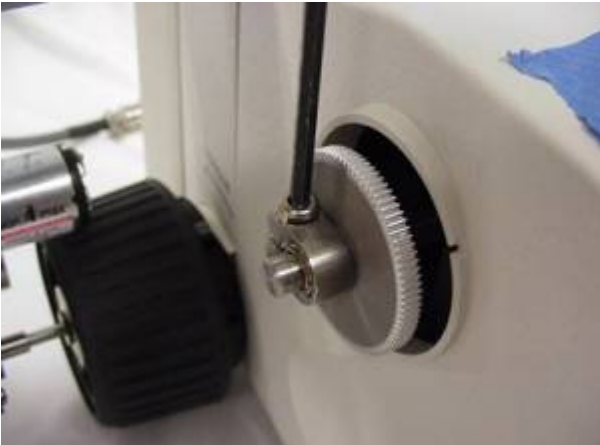
Figure 16. From the end of the zoom gear there should be a distance of 3/16 " (~ 4.5 mm) to the end of the shaft. Install & tighten the clamp as shown to secure the gear in place
