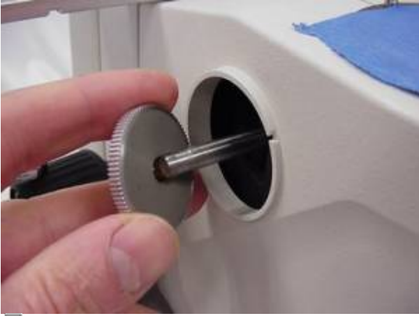
Figure 15. Installing zoom gear & spacer onto zoom shaft
