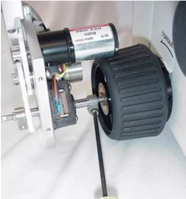
Figure 12. Push drive clamp up against focus knob & tighten
