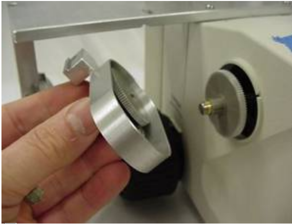
Figure 18. Install motor and cover gears need to mate.
