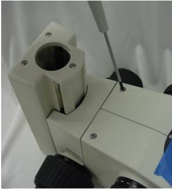
Figure 4. Use the cross blade screw driver to remove the two screws as shown
