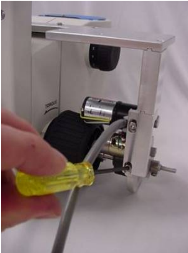
Figure 13. Tighten the vertical adjustment screws
