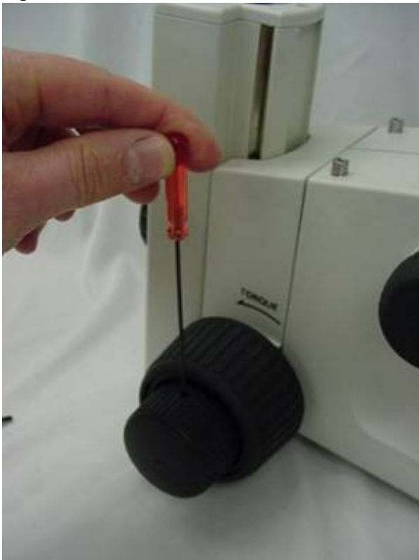
Figure 1b remove left fine focus & zoom knobs
