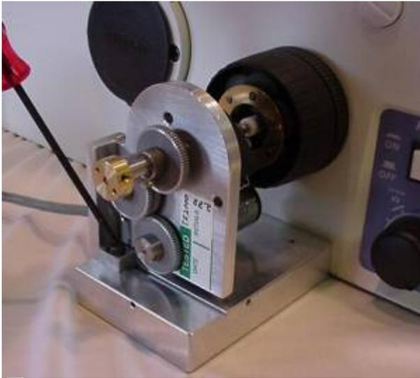
Figure 9 Horizontal Adjustment screw
