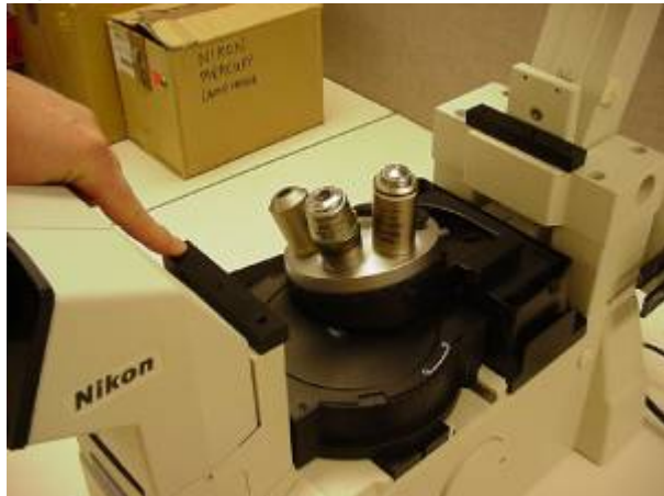
Figure 1. 12.75 mm stage spacers and 4ea. 5x25mm screws are required to mount the stage. On newer stages the spacers are attached to the stage.
