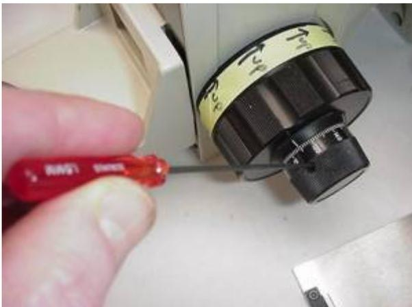
Figure 1: Use 1.5 mm Allen to loosen set screw
