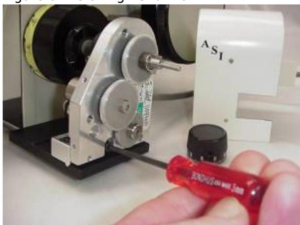
Figure 7. Installing vertical adjustment screw
