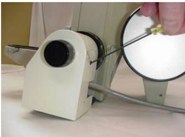
Figures 12: Installing cover and focus knob
