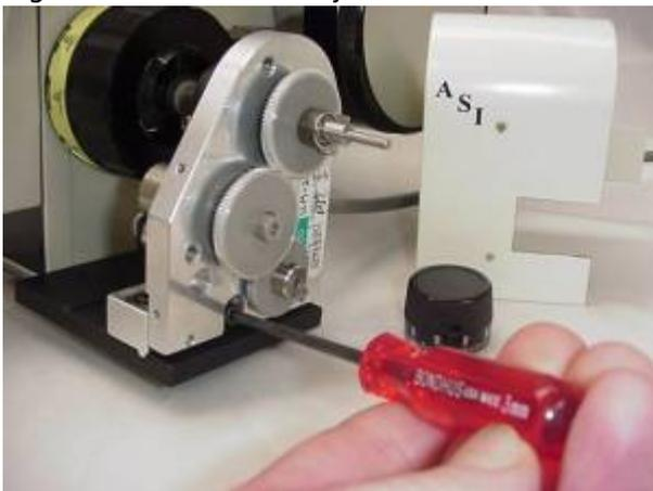
Figure 10: Vertical Adjustment screws
