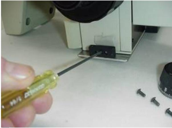
Figure 11: Tighten Baseplate set screw
