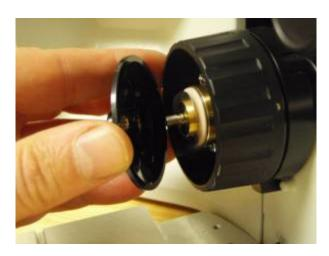
Remove the left fine focus knob from the microscope as follows:
