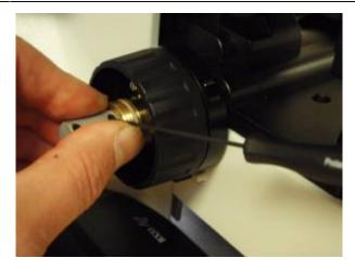
Locate the brass clutch plate and securely screw it on to the fine focus shaft. When installing the clutch insure that it is pressed all the way against the wave washer without pushing the right focus knob out at all. Check for any play in the focus shaft by pushing & pulling the right focus knob – there should be no play. Install the flex coupler as shown & fasten the flex coupler using a 1.5 mm Allen wrench.
