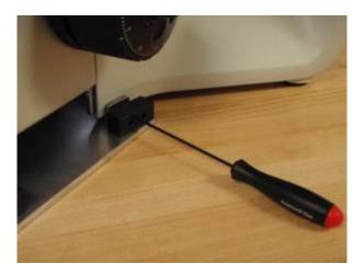
Use the 1.5 mm Allen wrench to tighten the base plate clamps as shown above.
