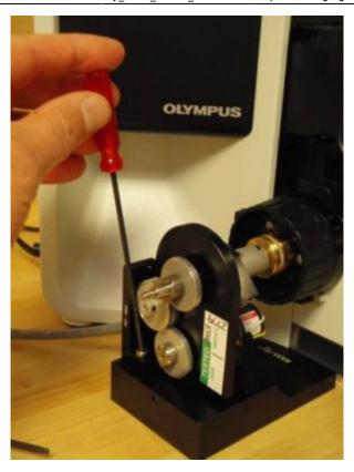
Slide the motor drive up and down, forward and backward slightly while turning the right fine focus knob until it is in the position where minimum drag is felt on the right focus knob. Secure the motor drive into position by tightening the horizontal and vertical adjustment screws
