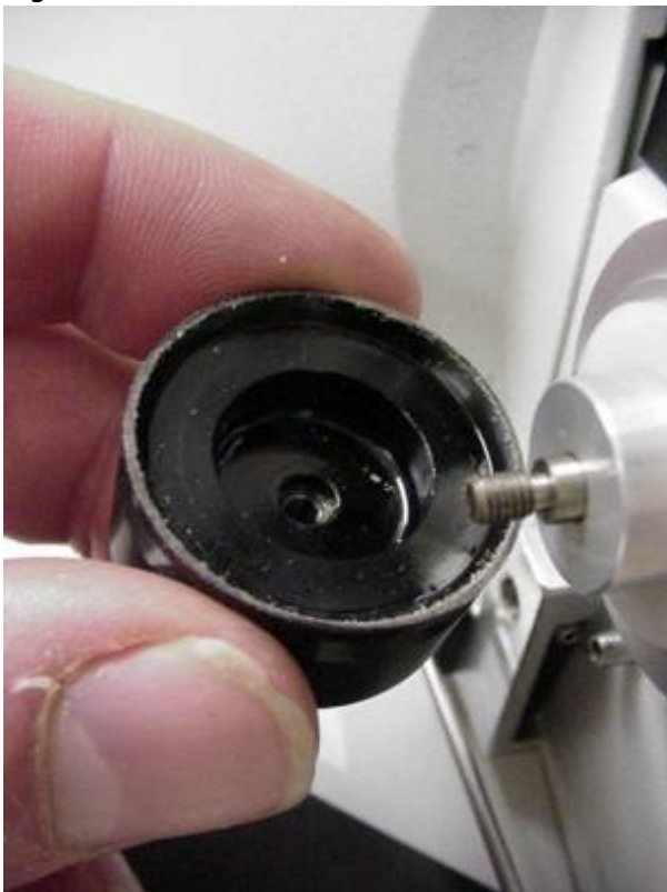
Figure 4. Hold on to right fine focus knob and unscrew the left fine focus knob
