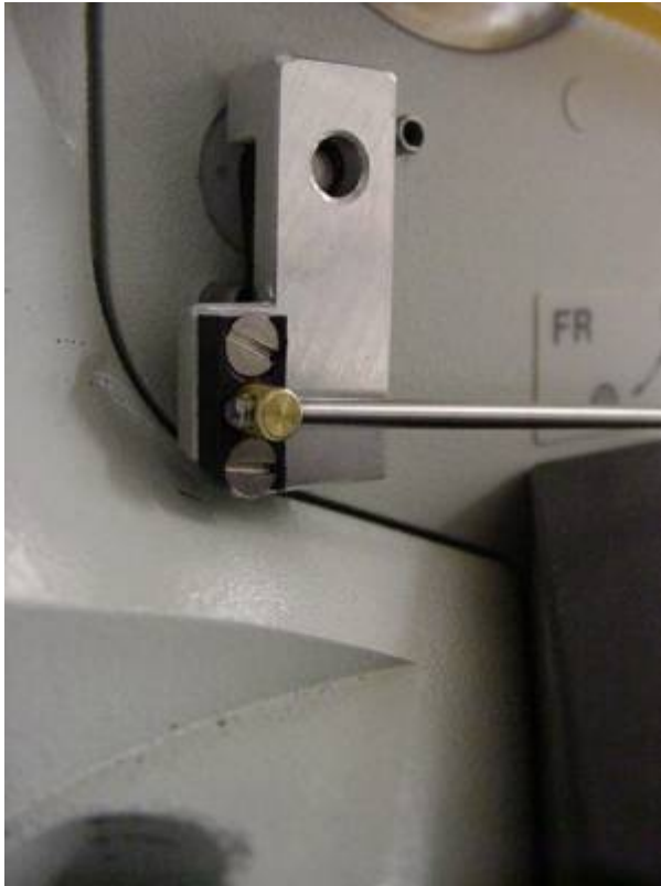
Figure 12. Diffuser switch extender installed.
