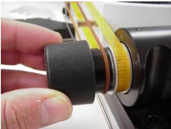
Figure 1. Pull rubber knob off of front focus knob
