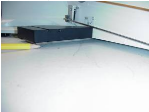
Figure 8. Baseplate needs to be mounted flush with the bottom of the microscope as shown. There should be a small gap between the bottom of the baseplate and tabletop.
