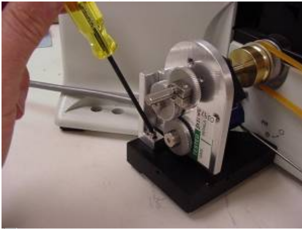
Figure 19. Check for alignment as outlined in the paragraph below, and then secure the horizontal ( as shown here), and the vertical adjustment screws as shown in figure 20.
