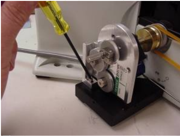
Figure 19. Check for alignment as outlined in the paragraph below, and then secure the horizontal ( as shown here), and the vertical adjustment screws as shown in figure 20.
