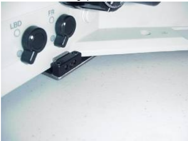
Figure 9. While holding baseplate in place against the bottom and the side of the microscope use the 5/64" Allen wrench to tighten the clamp on the right side of the baseplate.
