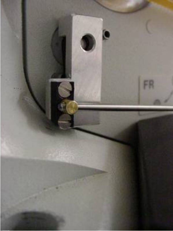
Figure 12. Diffuser switch extender installed.
