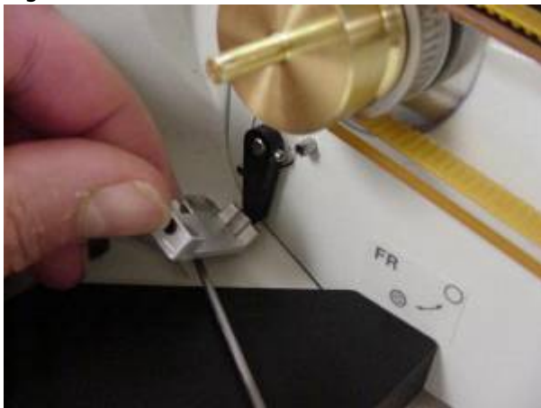
Figure 11. Installing diffuser switch extender. Use the 0.05 inch Allen wrench to tighten the set screw to hold the unit in place.
