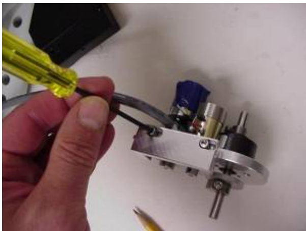
Figure 14. Use the 7/64" Allen wrench to loosen, but do not remove, the two vertical adjustment screws
