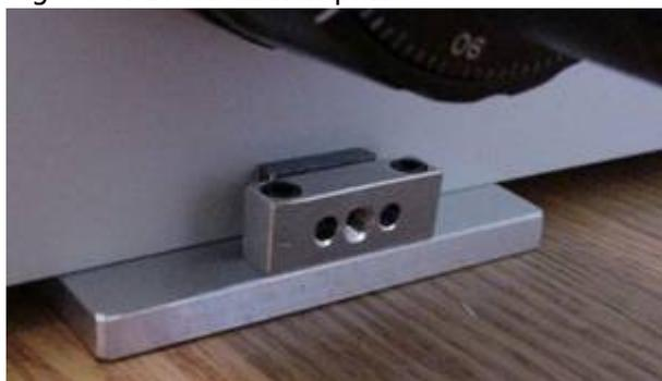
Figure 4. Base plate clamp assembly
