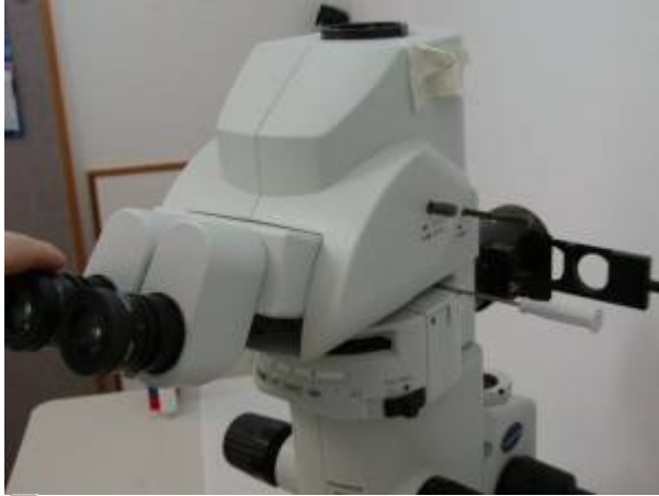
Figure 1 Remove the Objectives, Trinocular head & Fluorescence illuminator to reduce weight when installing the drive assembly. If necessary, please refer to the Olympus manuals for this microscope.
