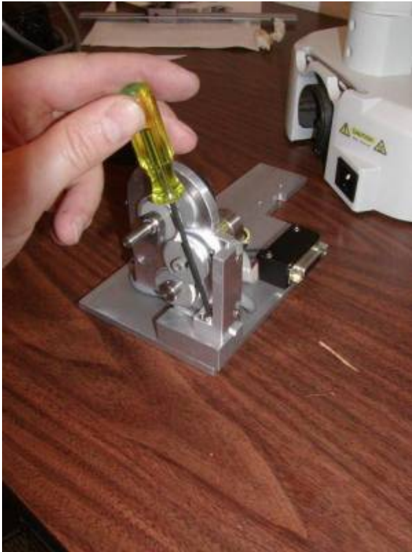
Figure 11. Loosening the horizontal adjustment screw
