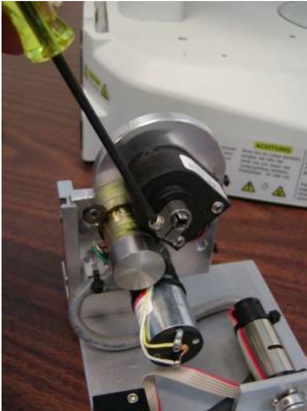
Figure 13. Loosening the drive shaft clamp
