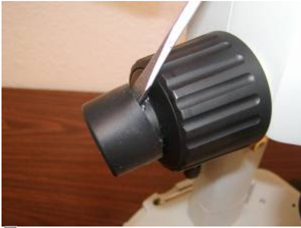
Figure 2 remove the rubber boot off of the end of the left fine focus knob
