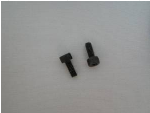
Figure 14. The two 4 x 10 mm screws that secure the base plate to the microscope.
