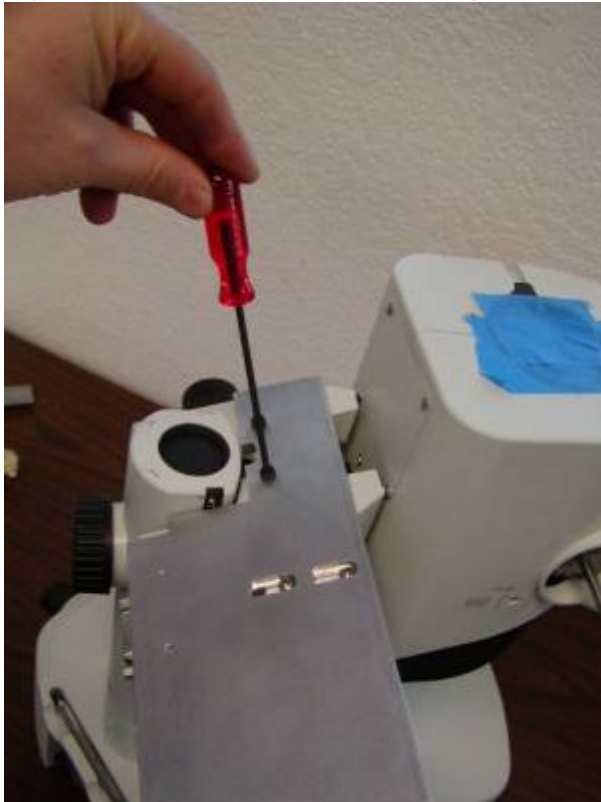
Figure 16. Use the two 4x 10 mm socket head cap screws to secure the base plate to the microscope
