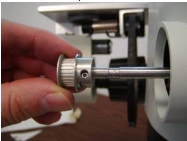
Figure 19. Use the 1.5 mm Allen wrench to loosen the two setscrews that secure the left zoom knob on to the microscope & remove the knob.
