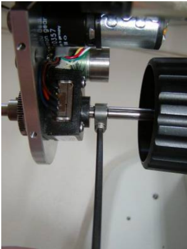
Figure 17. Use the 7/64" Allen wrench to tighten the drive shaft clamp. Please note: clamp must be
