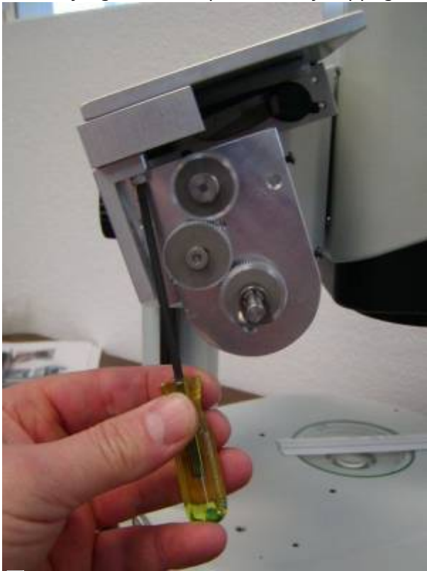
Figure 18. After tightening the drive shaft clamp as shown in figure 17, tighten the vertical and horizontal adjust adjustment screws
