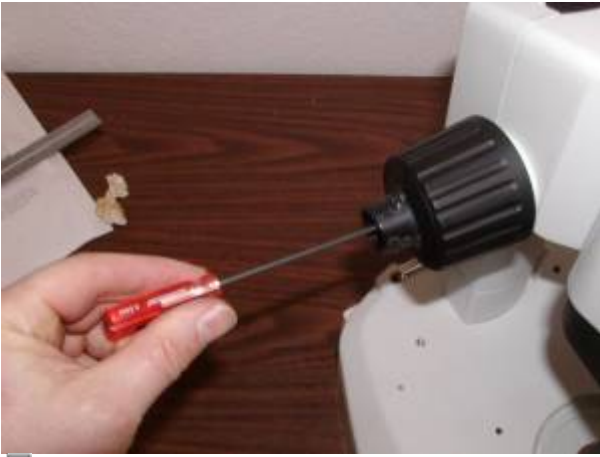
Figure 3 Location of Allen head screw to remove with 2.5 mm Allen wrench
