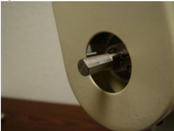
Figure 28. Flat on drive shaft that one setscrew from knob should mate with.
