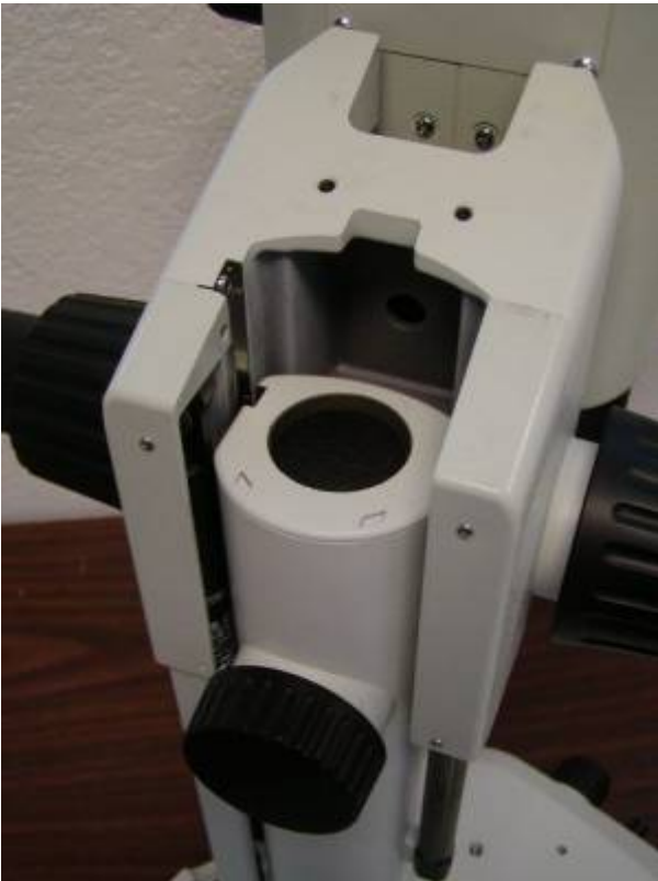
Figure 4. The focus assembly will rise up when the ffk is removed.
