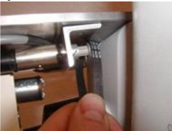
Figure 22. Install the zoom drive belt onto the motor & zoom shaft gears
