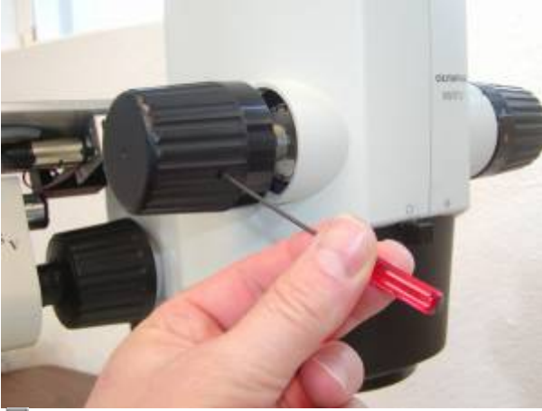
Figure 25. After installing the belt reinstall the zoom knob as shown.
