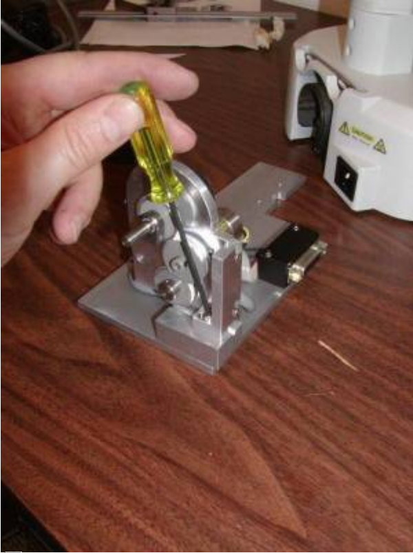
Figure 11. Loosening the horizontal adjustment screw
