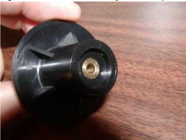
Figure 4. The focus assembly will rise up when the ffk is removed.
