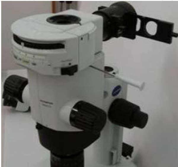
Figure 1 Remove the Objectives, Trinocular head & Fluorescence illuminator to reduce weight when installing the drive assembly. If necessary, please refer to the Olympus manuals for this microscope.
