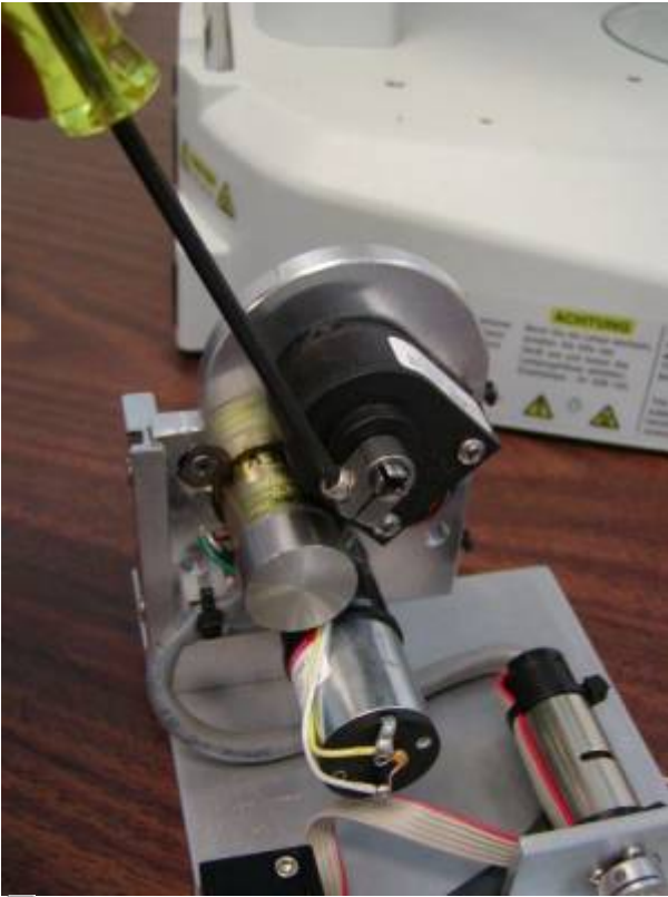
Figure 13. Loosening the drive shaft clamp
