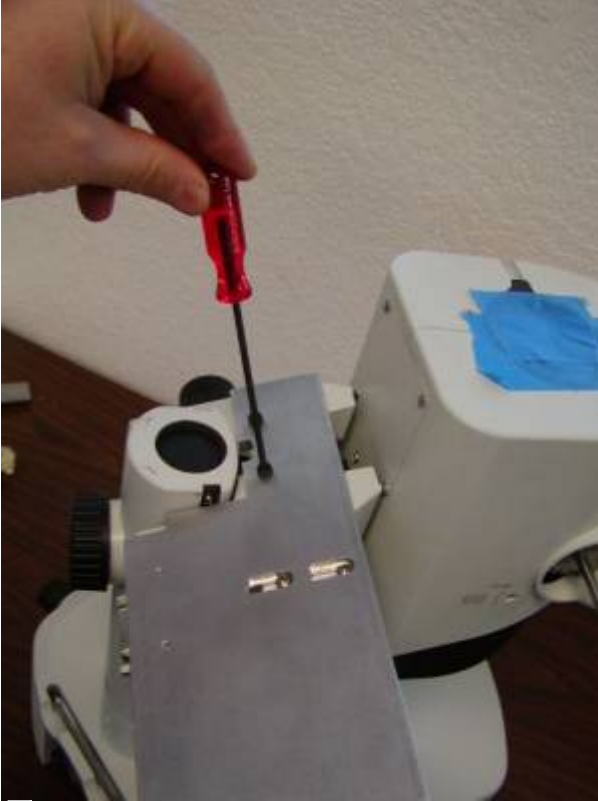
Figure 21. Use the cross blade screwdriver to loosen the two zoom motor adjustment screws.
