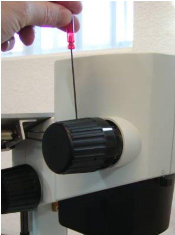
Figure 19. Use the 1.5 mm Allen wrench to loosen the two setscrews that secure the left zoom knob on to the microscope & remove the knob.
