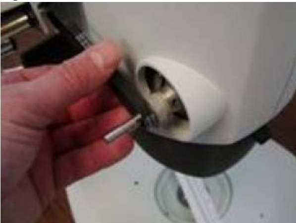
Figure 22. Install the zoom drive belt onto the motor & zoom shaft gears
