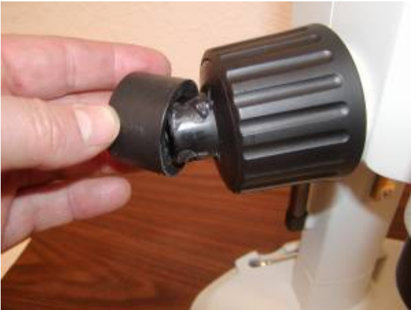
Figure 1 remove the rubber boot off of the end of the left fine focus knob
