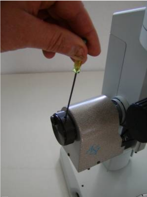
Figure 28b Install left focus knob as shown above. Make certain that one of the two setscrews from the knob mate with the flat on the drive shaft as shown. Use the 1/16" Allen wrench to tighten both set screws.
