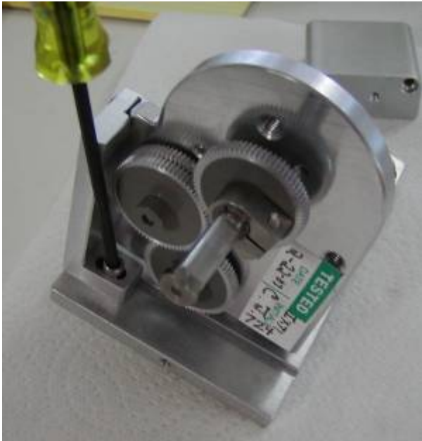
Figure 11. Loosen & remove the horizontal adjustment screw
