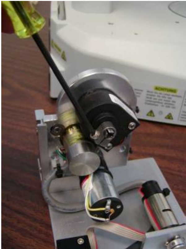
Figure 13. Loosening the drive shaft clamp
