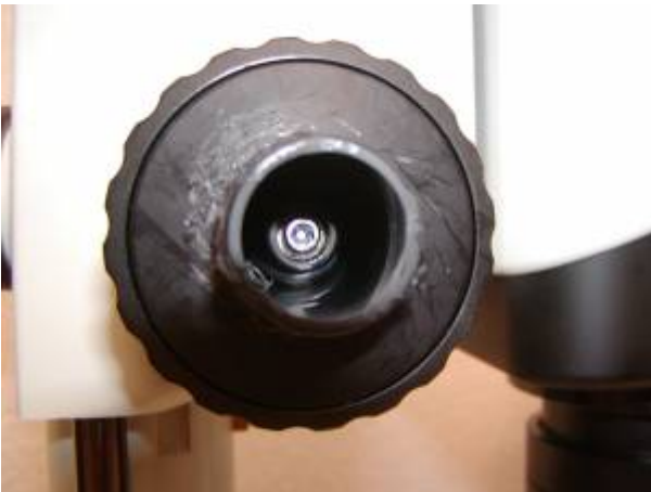
Figure 2 Location of Allen head screw to remove with 2.5 mm Allen wrench
