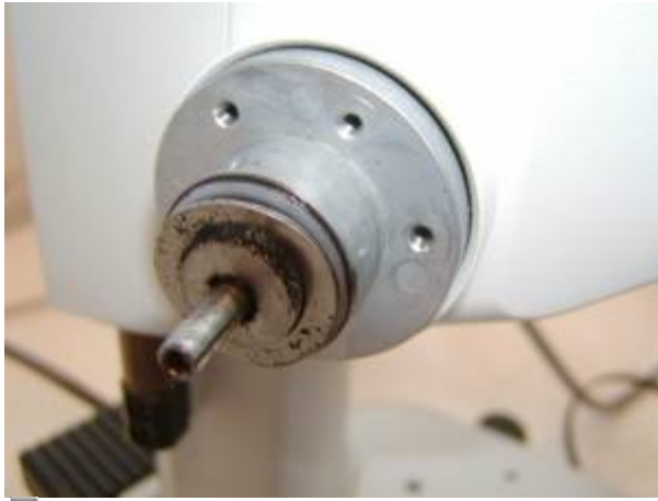
Figure 6. Use a cross blade screwdriver to loosen the three Philip head screws and remove the coarse focus knob as shown.
