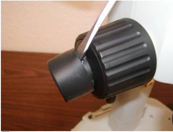
Figure 1 remove the rubber boot off of the end of the left fine focus knob
