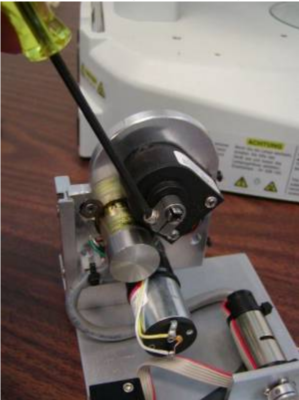
Figure 13. Loosening the drive shaft clamp
