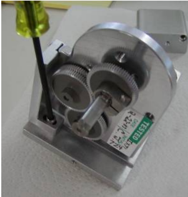
Figure 11. Loosen & remove the horizontal adjustment screw
