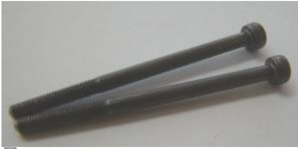
Figure 14. The two 3 x 45 screws that secure the base plate to the microscope.
