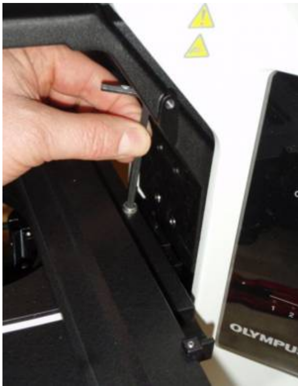
Location of rear stage mounting screw that uses the 5 x 12mm cap screw
