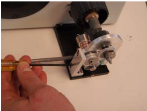
Tighten the vertical adjustment screws after alignment.
