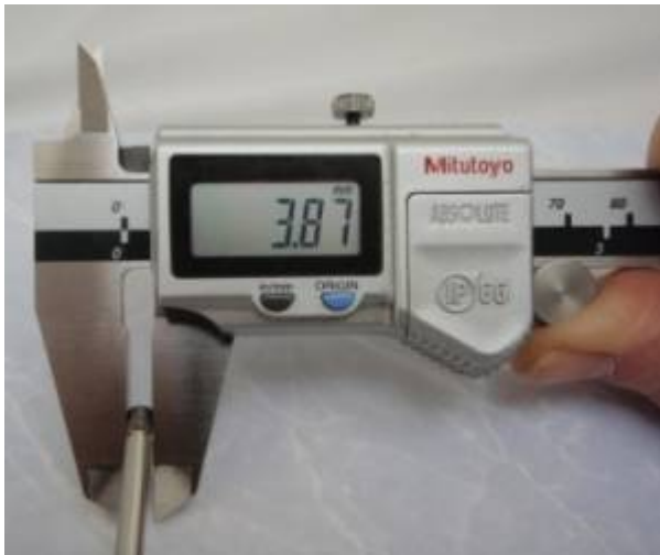
Typical diameter of threaded end of Olympus 4 mm fine focus shaft
