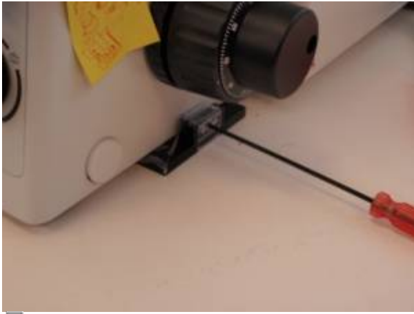
Tighten the baseplate clamp snugly.
