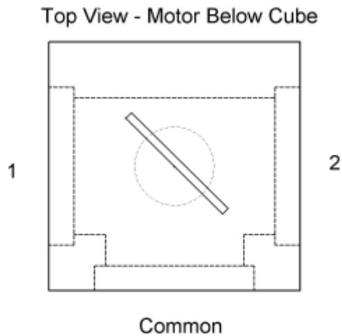
To set the mirror location for port 1 we need to have the illumination source connected to port 1 turned on and roughly focused at the objective BFP. Determine the name of the Port\_Switch axis. For the TIGER controller the [WHO](#) or [BU X commands](#) will reveal what is in the controller box. Below is an example where the port switch is named 'M' and is on card #2.
