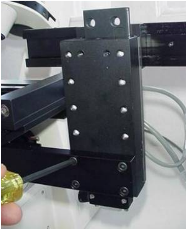
Fig 3c: attach LS50 to mounting bar
