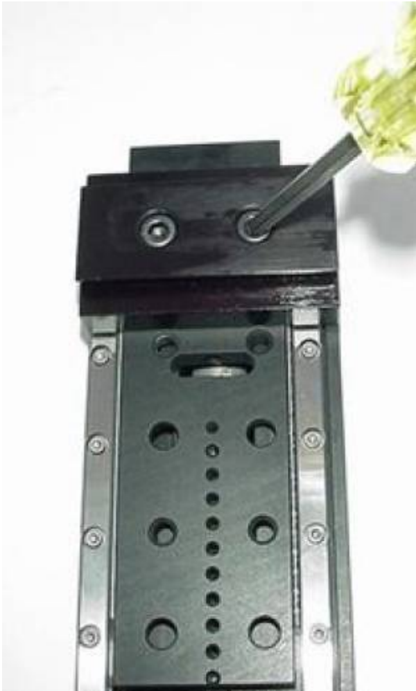
Fig 3b: attach male dovetail to LS50
