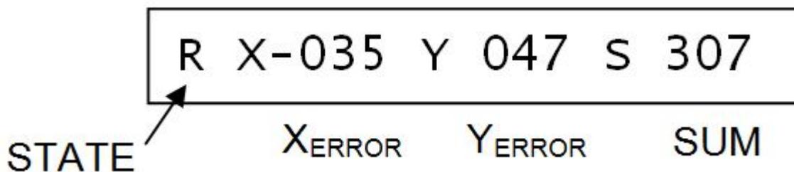
Figure 1: Bottom line of MS2000 controller's LCD. If you don't see this line , then Set Dip switch 2 in UP position.
