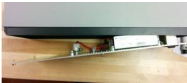
Figure 4: Pull out the back panel to access the power supply.
