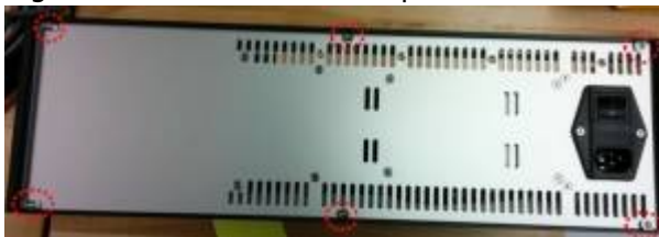
Figure 3: Location on Back panel screws on a TG-16 controller
