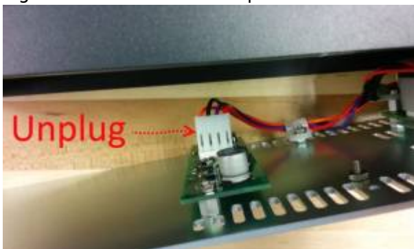
Figure 5: Unplug the Power supply connector
