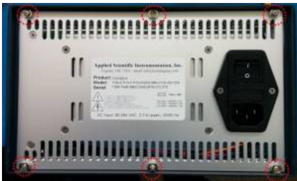
Figure 2: Location on Back panel screws on a TG-8 controller
