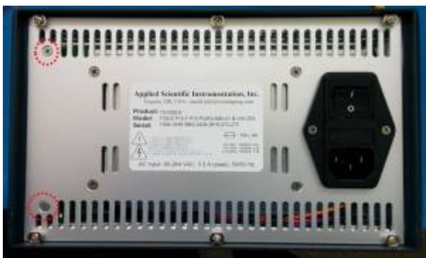
Figure 6: Location of Screws that hold power supply on Back panel in a TG-8 controller
