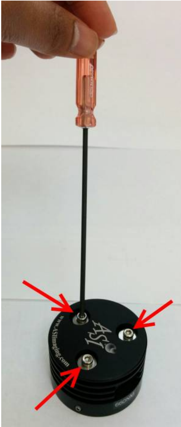
2.5mm Allen wrench to screw the three M2.5 screws
