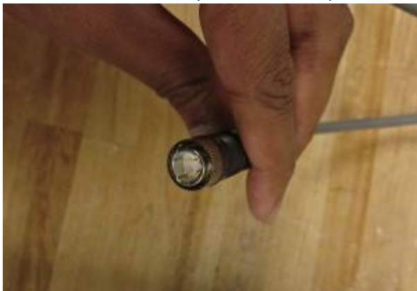
Insert's connector a 4pin HiRose connector
