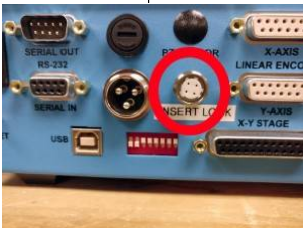
Corresponding connector on a MS2000 controller
