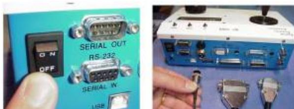
STEP 2: Remove the six case screws located on the back top and bottom front of the controller, (to avoid stripping screws when removing bottom screws, apply pressure to keep the top and bottom covers together while removing/inserting screws).
