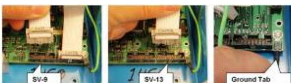
STEP 5: Get the new lid and find the same connections that were removed in step 4. They are labeled below. The connectors can be reattached to the case bottom in reverse order as in step 4.
