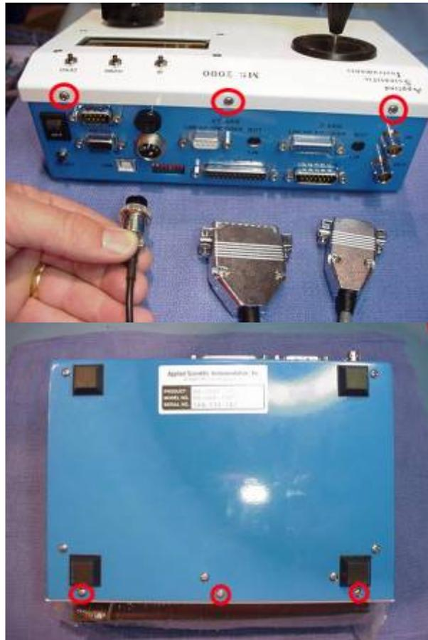
STEP 2: Remove the six case screws located on the back top and bottom front of the controller (to avoid stripping screws when removing bottom screws, apply pressure to keep the top and bottom covers together while removing/inserting screws).
